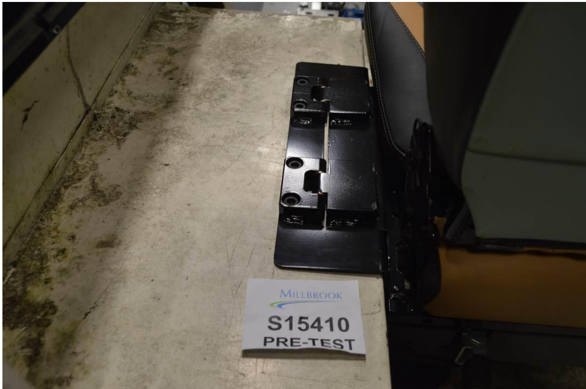
Rearward facing seat wheel arch mount, pre-test
