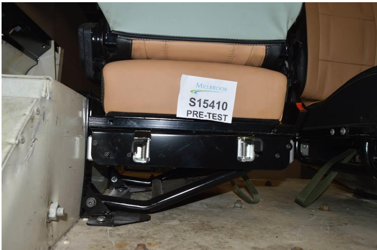
Rearward facing seat rear view, pre-test
